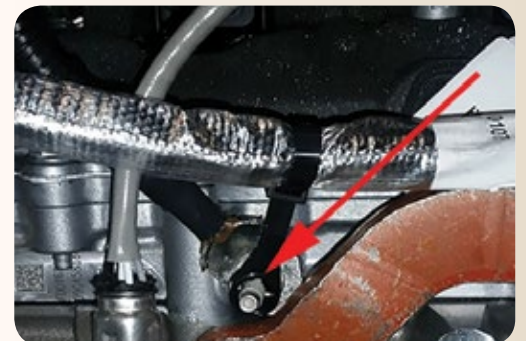
Loose ground connection
