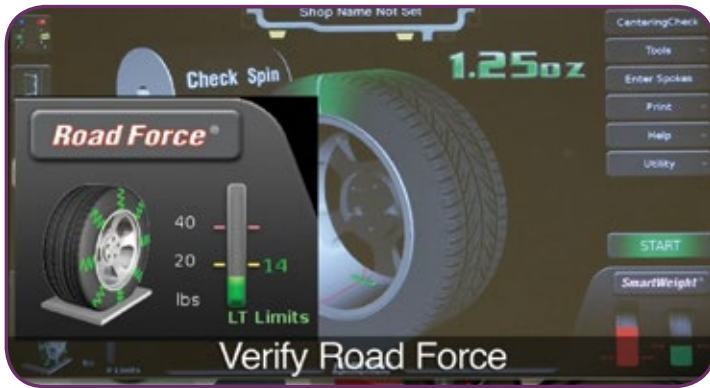
Use the Hunter Road Force Balancer to ensure tire/wheel assembly specifications are met.
