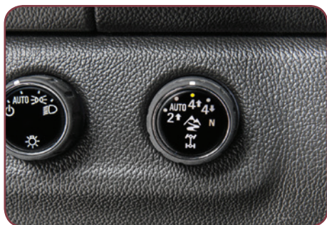
Transfer case knob with Off-Road Driving Mode control.
