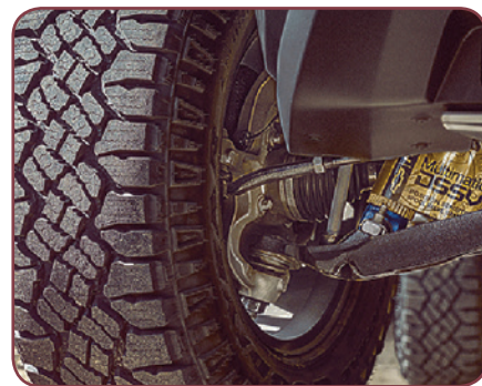
The Dynamic Suspensions Spool Valve (DSSV) damping system is tuned for a wide range of terrain.
