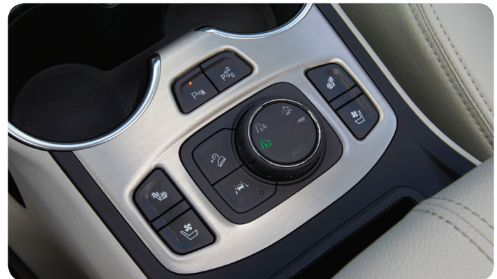
Switchable On-Off AWD control on the center console
