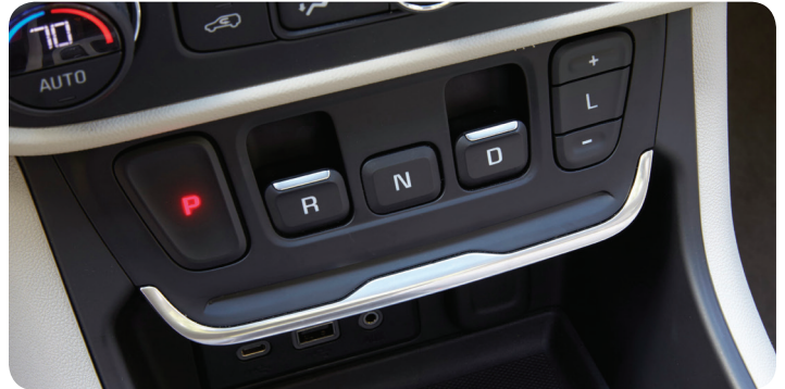
Electronic Precision Shift electronically-controlled gear selection
