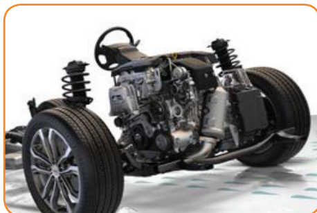
The Terrain has a MacPherson strut front suspension and a four-link independent rear suspension.
