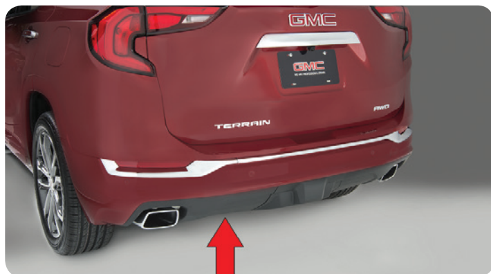
The location of the hands-free sensor is between the left exhaust pipe and the license plate.
