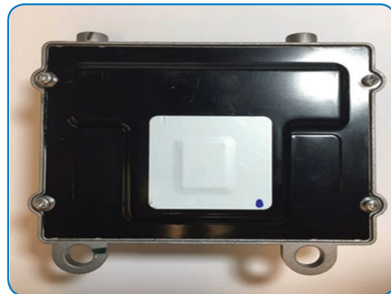
Look for corrosion between the base plate and the top housing.
