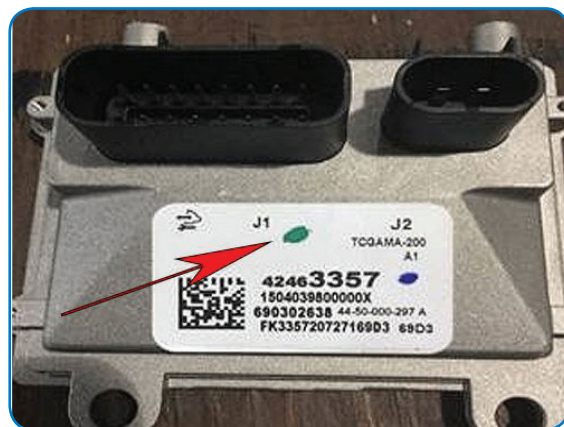
Only install a new module with a green dot on the part label.
