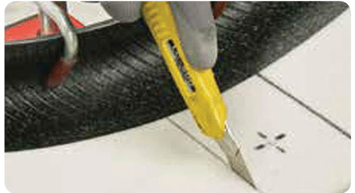
Remove a piece of foam 101 mm (4 inches) wide.
