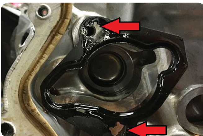
Gasket properly lined up to mounting bolt holes
