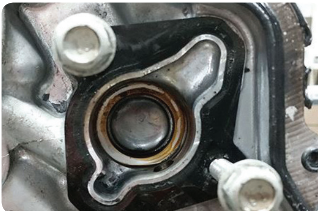
Correctly installed gasket
