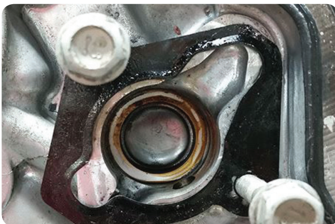
Incorrectly installed gasket
