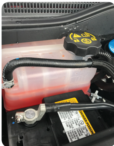
Low coolant level that will turn on the Low Coolant message.
