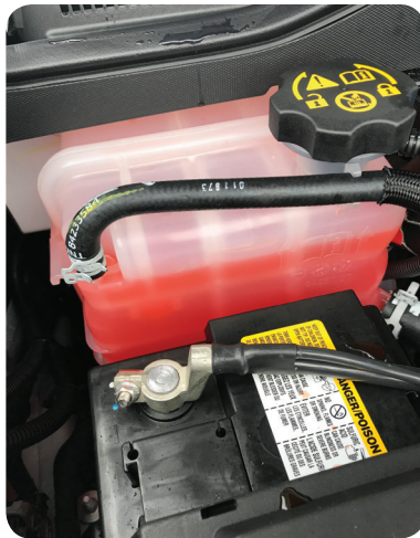
Coolant level at PDI. Coolant should be added to the surge tank when coolant is at this level.
