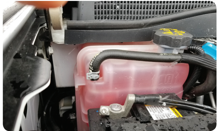
A full coolant level in the surge tank.
