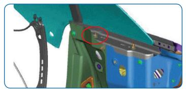
Loosen the forward nut to push out the base of the rear quarter glass.
