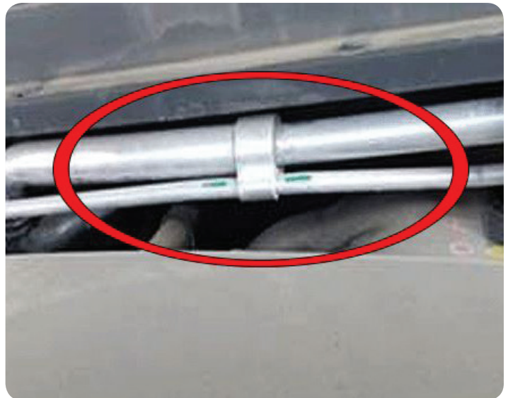
Clean the line using a soft wire brush.
