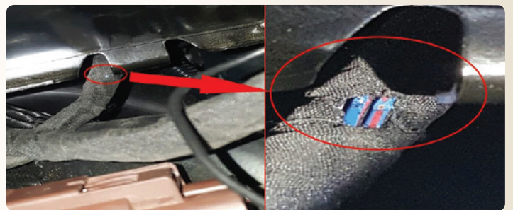
Harness damage at the battery tray
