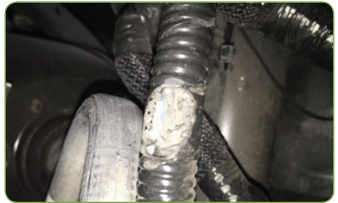
Harness rubbing on A/C pipe
