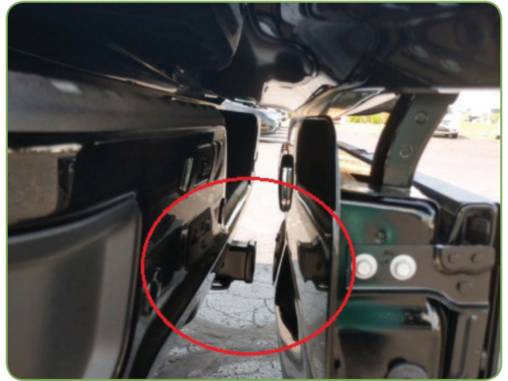
Clearance between hitch receiver and lowered inner gate.
