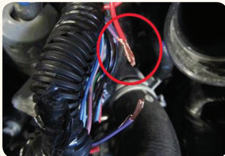
The repair used the largest gauge red wire and largest gauge purple wire.
