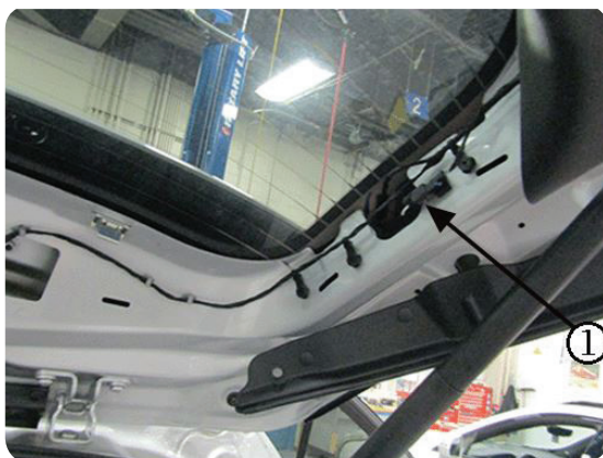
Remove the liftgate upper center and upper side trim panels to access the connectors.
