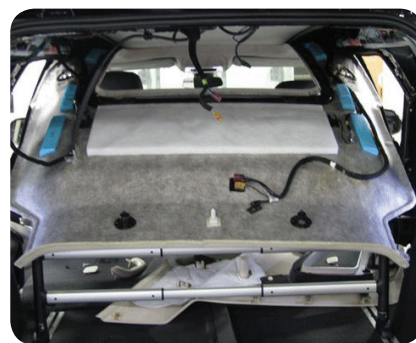
Lower only the rear portion of the headliner.
