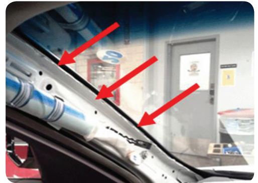
Observe the interior A-pillar for any evidence of water.
