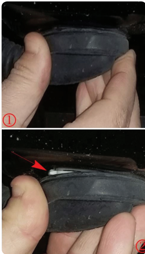
1. Properly seated grommet 2. Gap between the grommet and sheet metal
