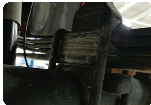
Slide the shim under the spring.
