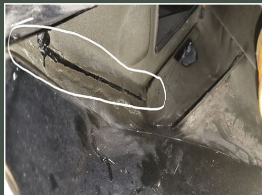
Apply sealer to the entire seam.
