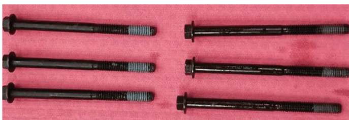
New bolts (left) and removed bolts (right)
