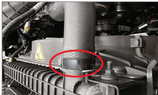
Coolant heat shrink hose clamp
