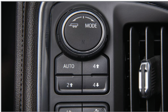
Autotrac system controls
