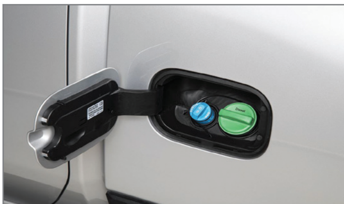
DEF filler is located next to the fuel filler.
