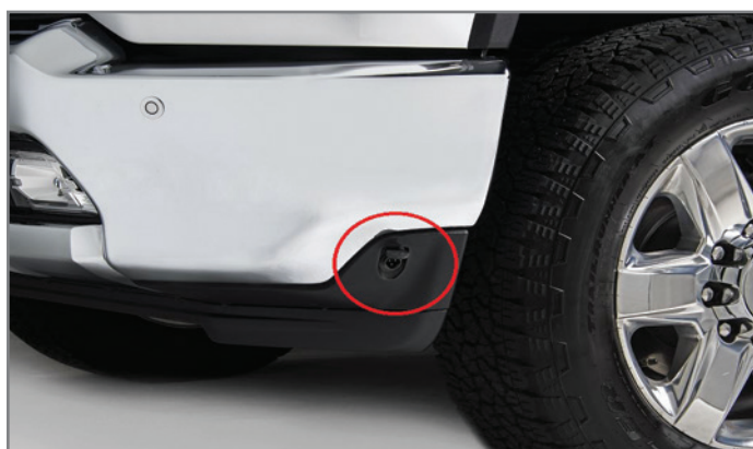
The engine coolant heater outlet is integrated into the front bumper.
