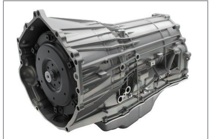
Transmission case with integral bell housing
