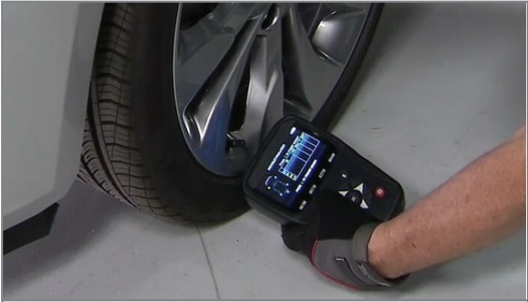
Place the front edge of the tool against the tire at the valve stem to relearn the sensor.
