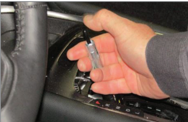
Clean the Park Switch electrical contacts by depressing the actuation rod 50 times.
