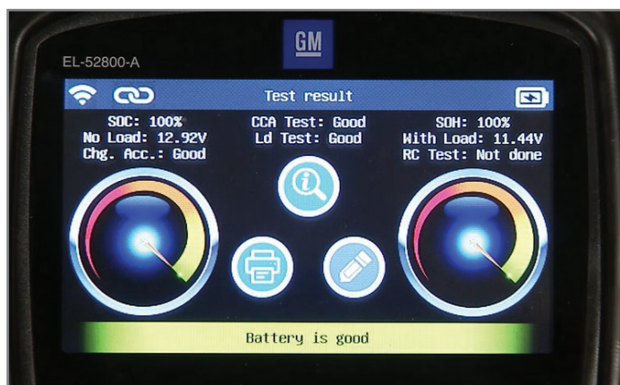
The on-screen results show if the battery is good or bad.
