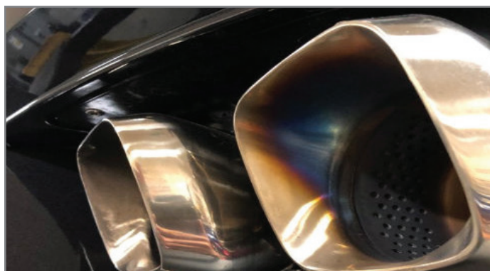
Bluing exhaust tips are a normal condition under high exhaust temperatures.
