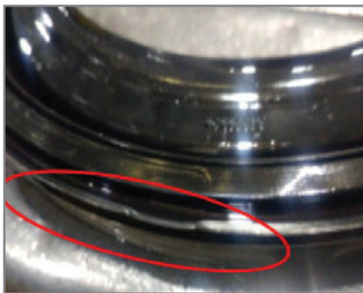
Rough finish on the center support housing may damage the Low-Reverse piston seal.
