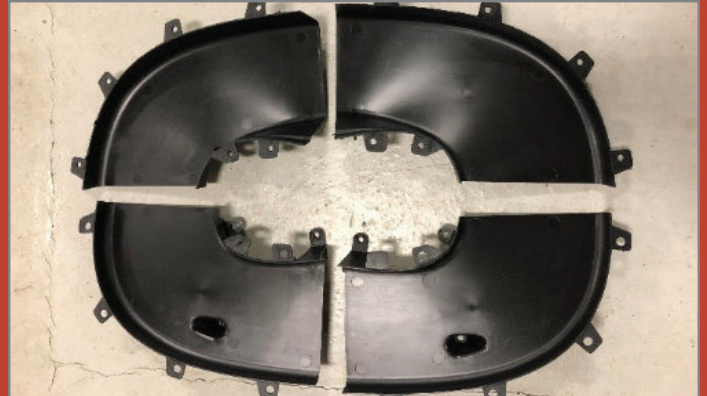
Rear control arm brake cooling ducts
