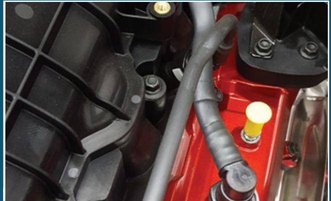
Incorrectly routed PCV tube
