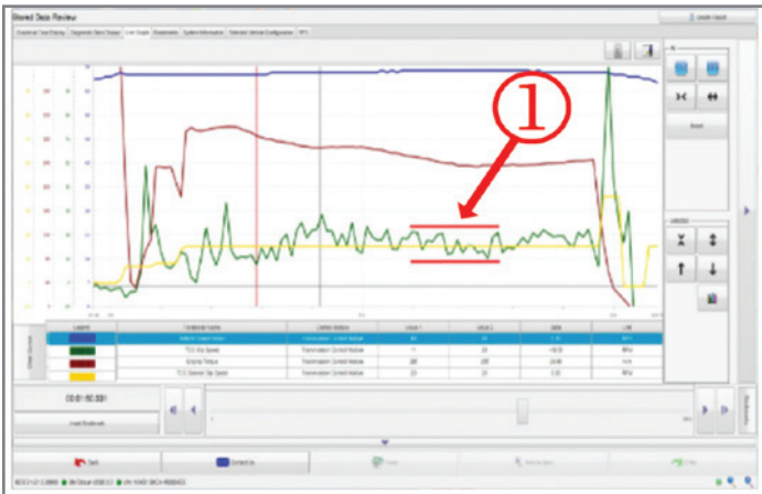
GDS2 data showing TCC slip peak-to-peak below 20 RPM.
