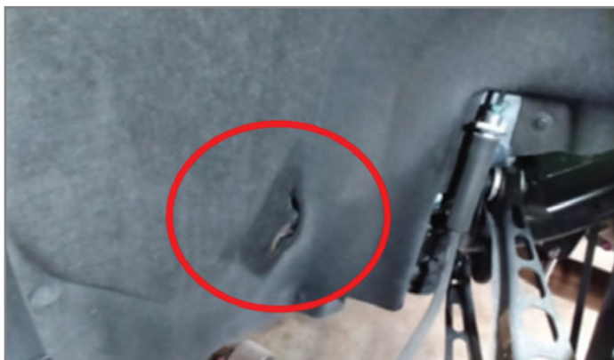
Rub-through on the left rear wheelhouse liner
