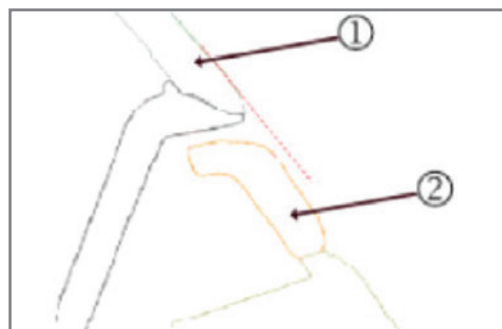
Dashed red line shows where the headlamp (#1) is proud of the fender (#2).
