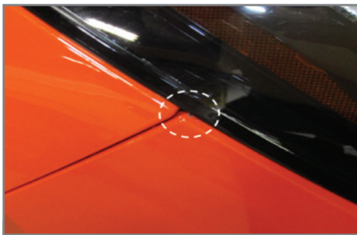
Paint chip in the front fascia
