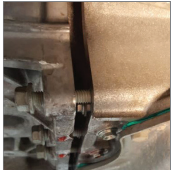
Slide the transfer case rearward so there is a minimum gap and then forward.
