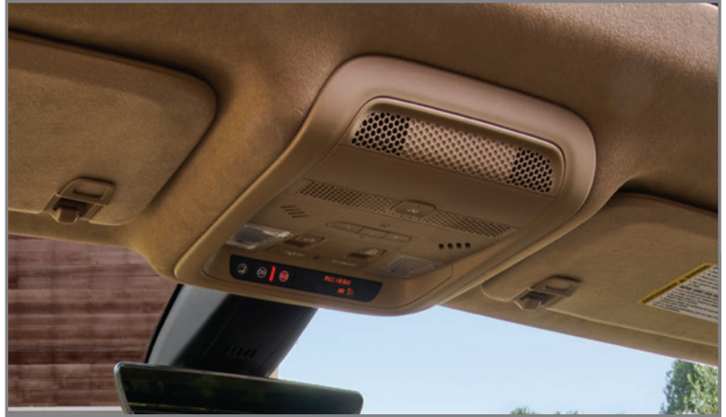
The Theft Deterrent Sensor is located in the overhead console.
