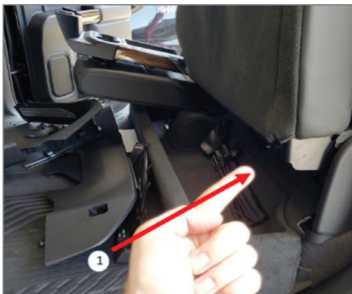
Check for a pinched body harness under the left rear seat.
