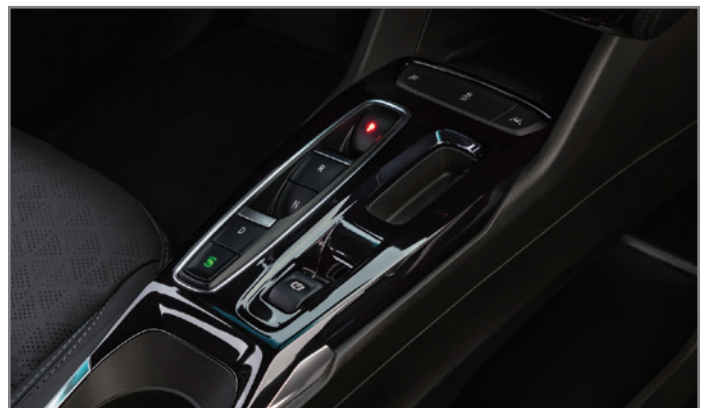
The electronic shifter features a push/pull switch operation.
