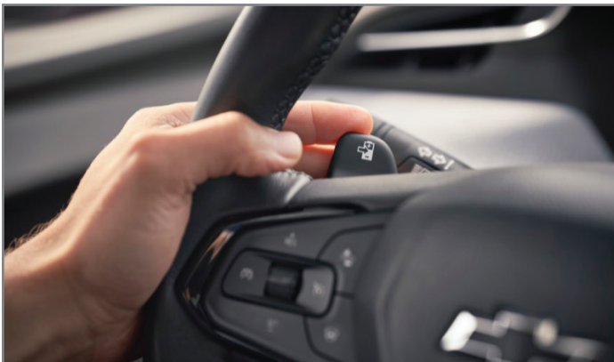
Regen on Demand paddle on the back of the steering wheel.
