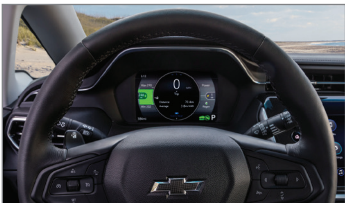
The instrument cluster layout can be changed using the right steering wheel controls.
