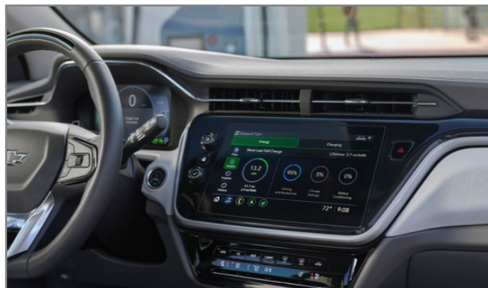
Energy graphics are displayed in the center stack energy screen, or “leaf screen.”
